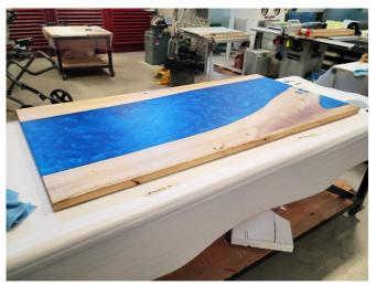
Figure 19: Table after 2 coats of Rubio Monocoat
