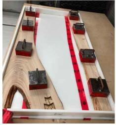
Figure 3: Test fitting wood slabs in mold
