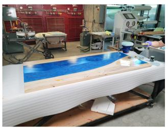
Figure 18: Application of Rubio Monocoat
