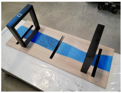
Figure 25: Coffee table with c-channel reinforcements
