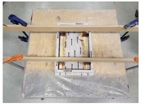
Figure 4: Using clamps and spacers to prevent slabs from moving
