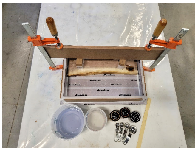
Figure 1: Work area and supplies for pouring
