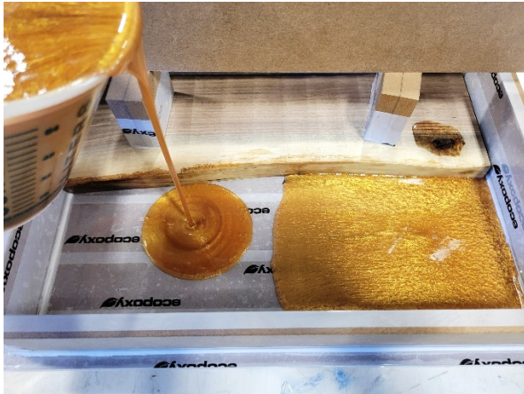
Figure 18: Pouring resin into the mold
