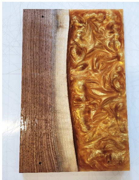
Figure 29: Oil applied to surface
